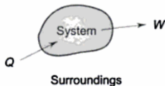
Fig. 4.3 Heat and work interactions of a system with its surroundings in a process
